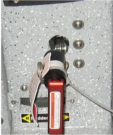
Fig. 2: New BRS rescue system handle installation which is not affected by this SD
