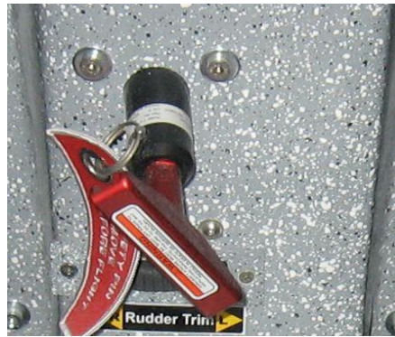
Fig. 1: BRS parachute system handle installation which is affected by this SD
